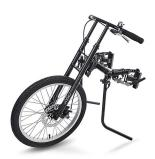
Extremely resilient aluminium frame in combination with stainless steel components ensures stability for very high strain.
